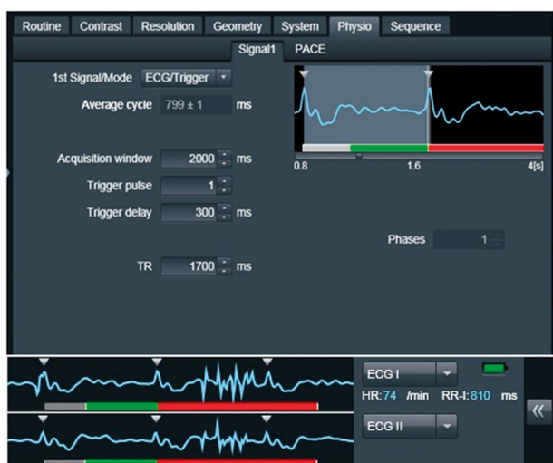
Figure 3. ECG-gating parameters used in acquisitions. Grey bar shows used delay of 300 ms
